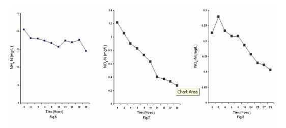
Fig 6-8: Performance evaluation of biosimulator (activated sludge treatment system) at 4.0 mg/L DO [Fig.6. NH<sub>3</sub>-N (mg/L); Fig.7. NO<sub>2</sub>-N (mg/L); Fig.8. NO<sub>3</sub>-N (mg/L)]
