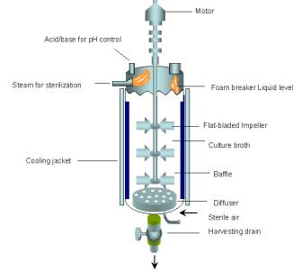
Fig 2 : General layout of a biosimulator (activated sludge treatment system)
