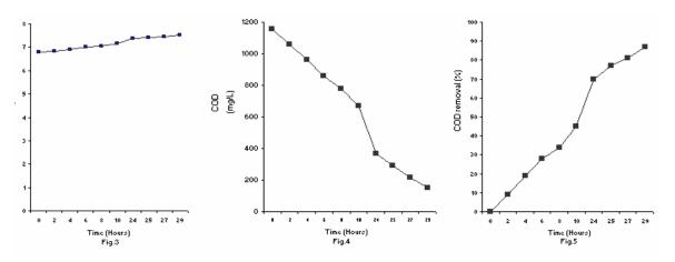
Fig 3-5: Performance evaluation of biosimulator (activated sludge treatment system) at 4.0 mg/L DO [Fig.3. Changes in pH values; Fig.4. Residual COD values; Fig.5. COD (5) removal efficiency]
