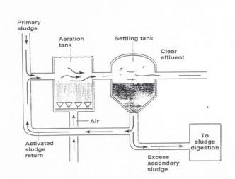
Fig 1. Sludge treatment system
