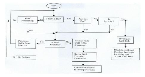
Fig 2. Flow chart for well producing at high HGOR
