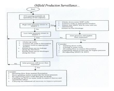
Fig 5. Flow chart for pressure surveillance
