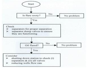
Fig 8. Surveillance for gas flares from flowstations
