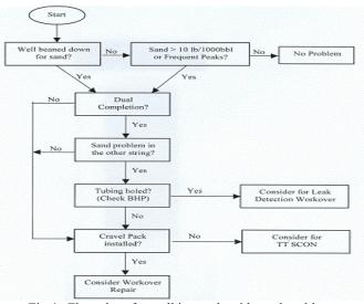
Fig 4. Flow chart for well intervals with sand problems
