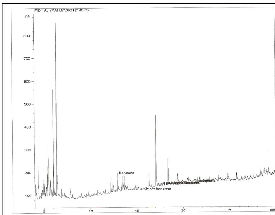
**Fig 2.** A chromatogram showing the distribution of BTEX in the impacted area
