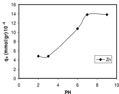
**Fig. 4-** Sorption isotherm of Zn<sup>2+</sup> ion on rice husks as a function of pH, 1g sorbent, 30mL of sample, temperature: 25±1 °C.
