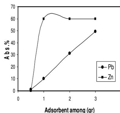
**Fig. 2-** Effect of sorbent dosage on the sorption of  $Zn^{2+}$  and  $Pb^{2+}$  on rice husks. Adsorption Conditions: 0.5-3g sorbent, 30mL of sample, pH 4.4, temperature:  $25 \pm 1$  °C.
