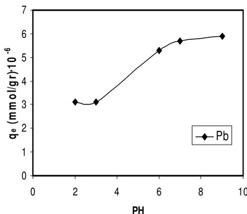
**Fig. 5 -** Sorption isotherm of Pb<sup>2+</sup> ion on rice husks as a function of pH/ 1g sorbent, 30mL of sample, °C.1temperature: 25±
