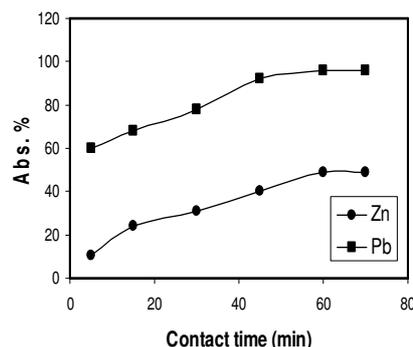
**Fig. 1-** Effect of contact time on the sorption of  $Zn^{2+}$  and  $Pb^{2+}$  by rice husks. Adsorption Conditions: 1g sorbent, 30mL of sample, pH 4.4, temperature:  $25 \pm 1$  °C.
