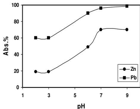
**Fig.3-** Effect of pH on the adsorption of Zn<sup>2+</sup> and Pb<sup>2+</sup> using rice husks. Adsorption conditions; 1 gr sorbent, 30mL of sample, temperature: 25±1 °C.
