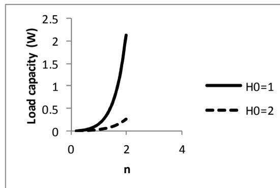
**Fig 5:** Variation of Load capacity with flow index for different values of  $H_0$  with  $\xi$  fixed at 10.0
