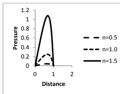
Fig 2: Variation of pressure with distance for different flow indices.
