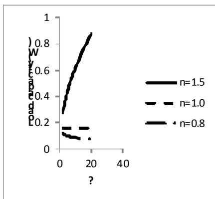
**Fig 4:** Variation of load capacity with  $\xi$  for different flow indices ( $n$ )
