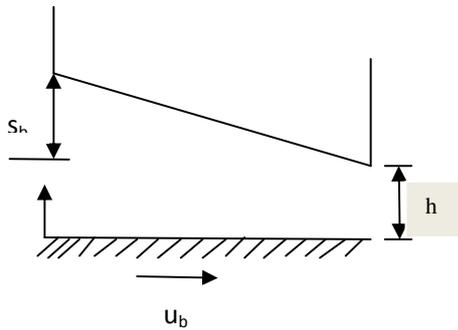
**Fig 1:** Geometry of a plane slider
