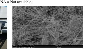
Fig 2. SEM image of quartz filter paper before sample collection
