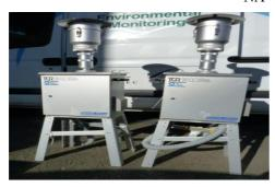
**Fig 1**. Tecora Echo high volume PM<sub>10</sub> sampler.
