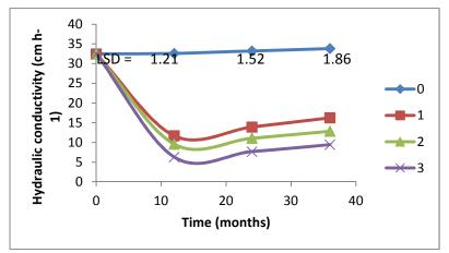
Fig 3: Effect of spent auto engine oil contamination on soil hydraulic conductivity (mean values)
