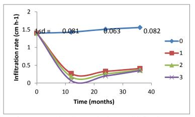
Fig 2: Effect of spent auto engine oil contamination on soil infiltration rate (mean values)
