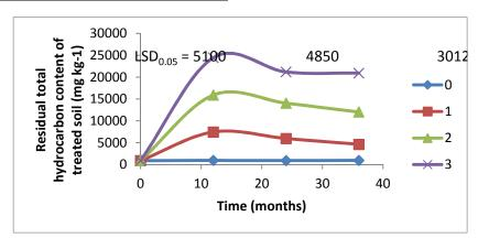
Fig 1: Changes in soil total hydrocarbon content (mean values) following spent engine oil loading
