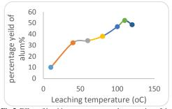
Fig 5: Effect of leaching temperature on the extraction of the alum (leaching time: 1.5 h; acid concentration: 4M; particle size:  $100 \ \mu m$ ,)
