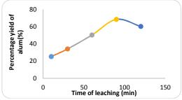
Fig 6: Effect of leaching time on the extraction of alum (acid concentration: 5M; particle size:  $100 \ \mu m$ ; temperature:  $110^{\circ}C$ )
