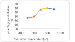
Fig 2: Effect of calcination temperature on the extraction of alum (time: 1.5 h, particle size: 100 µm)
