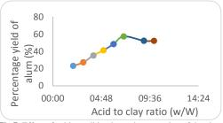
Fig 7: Effect of acid to solid ratio on the extraction of the alum (leaching time: 1.5 h; temperature: 110°C; particle size: 100µm; acid concentration: 5M)
