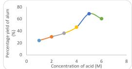
Fig 8: Effect of H<sub>2</sub>SO<sub>4</sub>concentration on the extraction of alum (leaching time:1.5 h; temperature:110°C; particle size: 100 µm)
