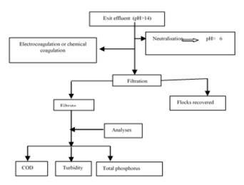
Fig 1. Illustration of the treatment procedure
