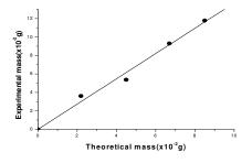
Fig 2: Variation of the experimental mass against the theoretical mass of aluminium during the treatment of textile effluent. Electrocoagulation time= 40 minutes.
