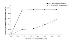
Fig 6: Effect of the quantity of Al<sup>3+</sup> on the total phosphorus removal during electrocoagulation and chemical coagulation of the textile effluent.
