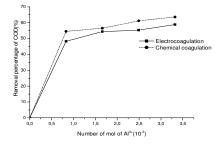
Fig 7: Effect of the quantity of Al<sup>3+</sup> on the COD removal during electrocoagulation and chemical coagulation of the textile effluent
