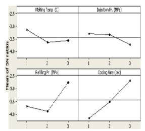
Fig 1: Plot of Main Effects for S/N ratio
