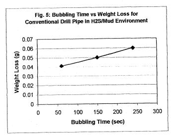
Corrosion Test for Drilling Mud (H<sub>2</sub>S)
