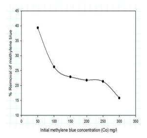
Figure 2. Effect of initial dye concentration on the removal of methylene blue using adsorbents from rice husk.
