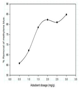
Figure 5: Effect of adsorbent dosage of rice husk on the removal of methylene blue
