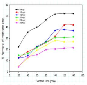
Figure 4: Effect of Contact time and initial methylene concentration on the removal of methylene blue using rice husk-based adsorbent.
