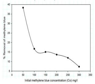
Figure 1. Effect of initial dye concentration on the removal of methylene blue using adsorbents from rice husk.
