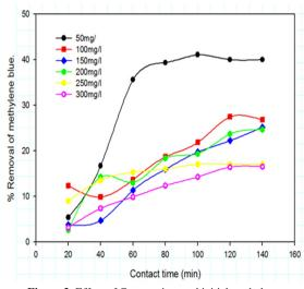
Figure 3: Effect of Contact time and initial methylene concentration on the removal of methylene blue using Coconut shell-based adsorbent.
