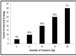
Fig 4: Quantity of fume produced with ANFO
