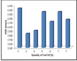
Fig 6: Quantity of Fuel Oil versus VOD
