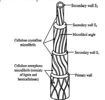
Fig 3: Structural components of natural fibre (Kabir et al., 2012)
