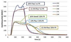
Fig 6. Heat release rate of PA 6 reinforced by different content of natural fibre and FR (Elsabbagh *et al.*, 2017).
