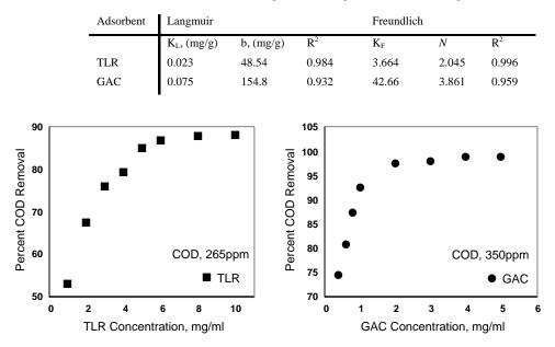
Fig 2. Effect of adsorbent concentration on COD removal by TLR and GAC
