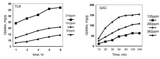
Fig 3. Kinetics of COD removal at various concentrations TLR and GAC
