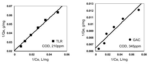
Fig 5. The linearized Langmuir Adsorption Isotherm for COD with TLR and GAC
