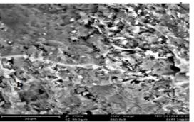
Fig 2b SEM Micrograph of residual coal(Treated) at 30µM
