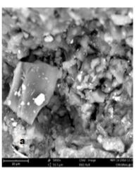
**Fig 1a:** SEM Micrograph for Virgin Coal at 10µM
