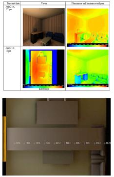
Fig 4: Normal analysis of illuminance level on work plane using lights cape software.
