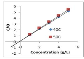
Fig 1: Langmuir plot for leaf in 1.0M H<sub>2</sub>SO
