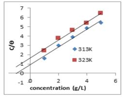
Fig 3: Langmuir plot for leaf extract in 5M H<sub>2</sub>SO<sub>4</sub>
