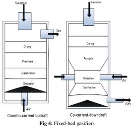
*Downdraft gasifier*: In a downdraft gasifier, air interacts with solid biomass in the downward direction, with the flow of wastes and gases in a cocurrent direction. All the decomposition products from the pyrolysis and drying zones are forced to pass through the oxidation zone for thermal cracking of volatile materials, producing a gaseous fuel with less tar (Chopra and Jain, 2007). Here, the air interacts with pyrolyzing biomass before making contact with char
