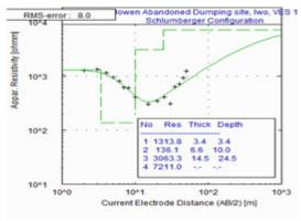
Fig 3a: Resist graph showing iteration for VES 1
