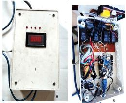
Fig 5: Smart switch prototypes: (A) Enclosed, (B) Opened to reveal components
