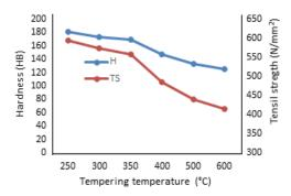
Fig 3: Hardness and Tensile strength at different tempering temperatures (previously quenched from 900°C)
