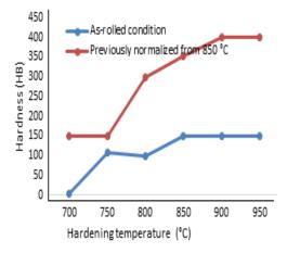
Fig 5: Hardness of the steel in the as-rolled condition and after normalization
