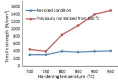
Fig 6: Tensile strength of the steel in the as-rolled condition and after normalization
