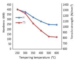
Fig 4: Hardness and Tensile strength at varying tempering temperatures (previously normalized and quenched at 850 °C)
