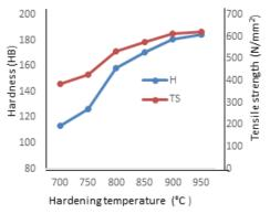
Fig 1: Effect of Hardening temperature on hardness and tensile strength without normalizing
