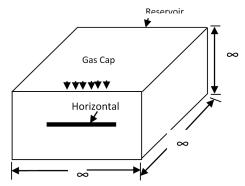
Fig 9: Reservoir Top Gas Cap and Infinite acting
