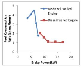
Fig 2. Variation of fuel consumption rate of the engine when it was run with biodiesel and diesel with brake power.
