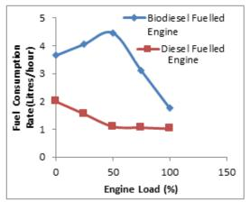
Fig 1. Variation of fuel consumption rate of the engine when it was run with biodiesel and diesel with engine load.
