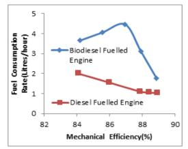
Fig 3. Variation of fuel consumption rate of the engine when it was run with biodiesel and diesel with mechanical efficiency.
