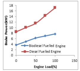
Fig 4. Variation of brake power of the engine when it was run with biodiesel and diesel with engine load.
