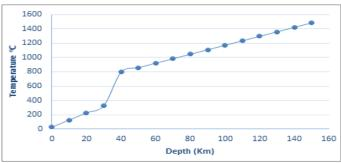
Fig 1: Temperature against Depth
