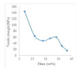
Fig 2: Tensile strength of composite at different weight percent
