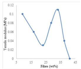
Fig 5: Tensile modulus of composite at different weight percent
