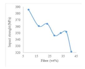
Fig 3: Impact test for composite at different weight percent
