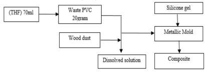
Fig 1: Schematic view of production procedure
