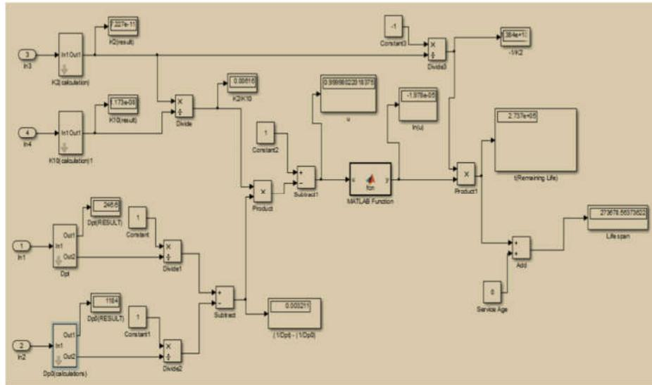
Fig 5: Complete Simulink Model for the Determination of Lifespan of a Power Transformer
