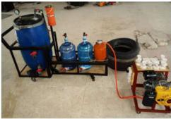
Fig 7: Biogas production, purification and power generation system
