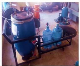
Fig 5: Biogas production and purification system
