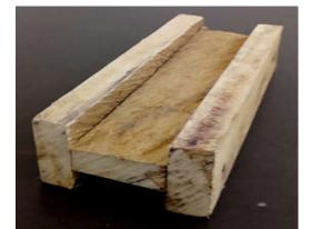
Plate 1 Showing I-Section Test SpecimenThe limit state or performance function incompression as given by (Nowak and Collins 2000) $g(x) = f_{p \ par} - f_{a \ par}$ .(1)
