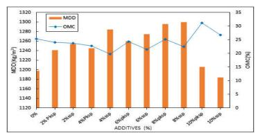
Fig 1. Compaction characteristics of the soil stabilized with varying PKSP and SSP.
