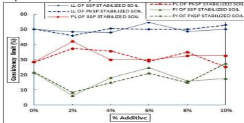
Fig. 3. Consistency behaviour of the soil stabilized with varying PKSP and SSP.
