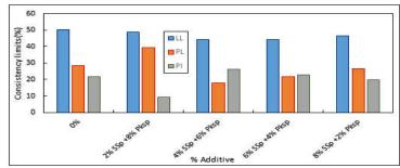
Fig. 4. Consistency behaviour of the soil stabilized with combined PKSP and SSP
