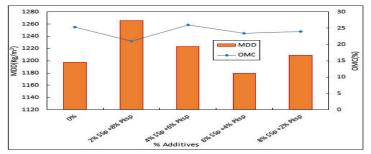
Fig. 2. Compaction characteristics of the soil stabilized with combined PKSP and SSP
