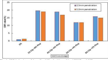
Fig. 6. CBR behaviour of the soil stabilized with combined PKSP and SSP
