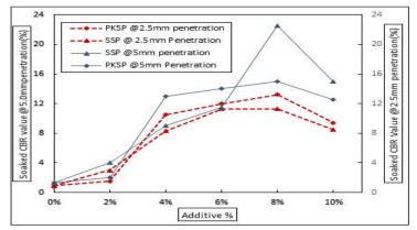
Fig. 5. CBR behaviour of the soil stabilized with varying PKSP and SSP
