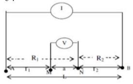
Fig 3: Schlumberger Field Electrode Configuration.
