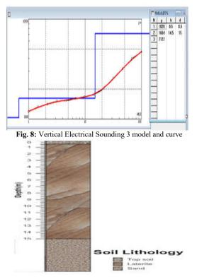
Fig. 9: Lithology of Vertical Electrical Sounding 3 interpretation
