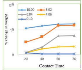
Fig 1: Graph of PVA/TPS Cast Film Absorption Rate in Toluene
