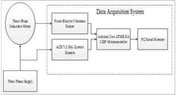
Fig 5. Data Acquisition Block Diagram
