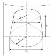
Fig 1: Stator Slot Surface
