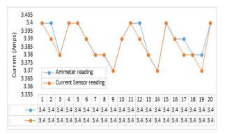
Fig 10: Current sensor validation
