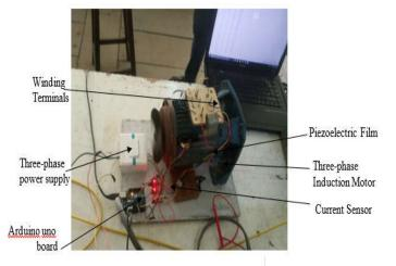
Fig 9: Experimental Test Rig
