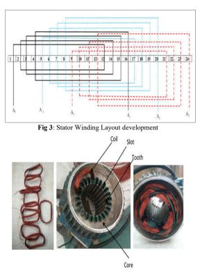
Fig 4: Inserting Formed Wound Coils in Stator
