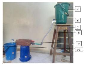
Fig 2. Magnetic treatment unit for the wastewater: Legend: 5 = Storage tank, 6 = control tap, 7 = stood, 8 = hose, 9 = magnetic field unit, 10 = collector for the wastewater
