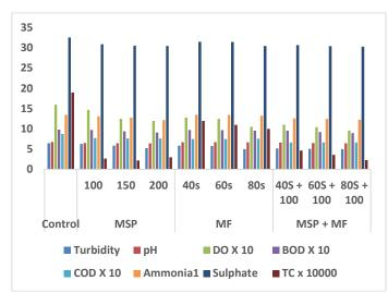
Fig 3. Results of physicochemical and total coliform (TC) in the wastewater before and after treatment MSP = Moringa seed powder at 100, 150 and 200 mg/L, MF = Magnetic field used in 40, 60 and 80 s
