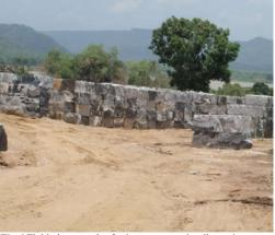
Fig 6.Field photograph of primary cut gneiss dimension stone migmatite parked before moving to secondary cutting and polishing plant.
