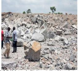
Fig 2. Field photograph of biotite granite blasted for production of aggregates at Kporokpo village.
