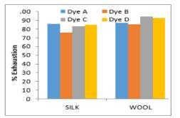
Fig 9. Effect of Type of fabric (silk & wool) on dye absorption at optimum temperature
