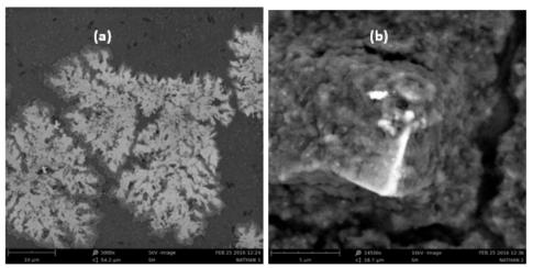
Fig 4a SEM of FeNPs and b is SEM of CuNP
