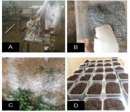
**Fig. 1:** Aluminum particles yield at a fabricator's workshop (A), collected Aluminum debris (B), soil contaminated with Aluminum particles in ambient environment (C), and five replications of control soil as well different concentrations of Aluminum spiked on soil in exposure vessels (D).
