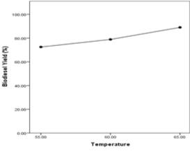
Fig 6: Effect of reaction temperature on biodiesel yield
