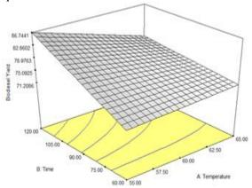
Fig 3: 3-D plot of yield with respect to temperature and time
