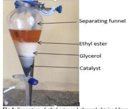
Fig 1: Separation of ethyl ester and glycerol obtained from transesterification process
