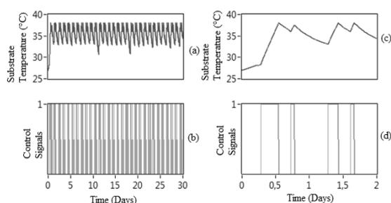
**Fig 7 :** Substrate temperature and Control signals for 3,000Kg of organic matter
