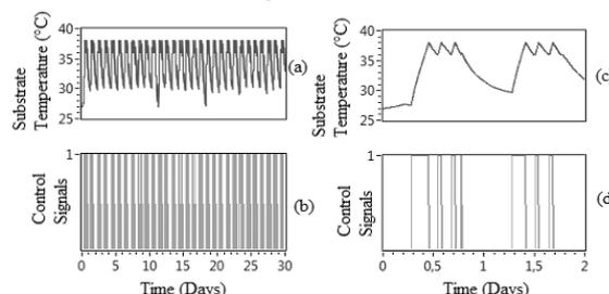
**Fig 5 :** Substrate temperature and Control signals for 1,500Kg of organic matter
