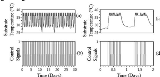
**Fig 3 :** Substrate temperature and Control signals for 500Kg of organic matter
