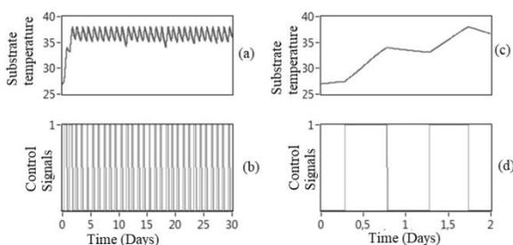
**Fig 8 :** Substrate temperature and Control signals for 10,000Kg of organic matter
