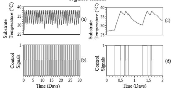
**Fig 6 :** Substrate temperature and Control signals for 2,000Kg of organic matter
