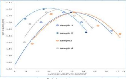
Fig 3: Compaction curves
