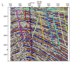
Fig. 4: The vertical section through ATA 11 showing the faults and mapped horizon
