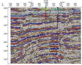
Fig. 3: Seismic section showing synthetic seismogram tying with well ATA 11
