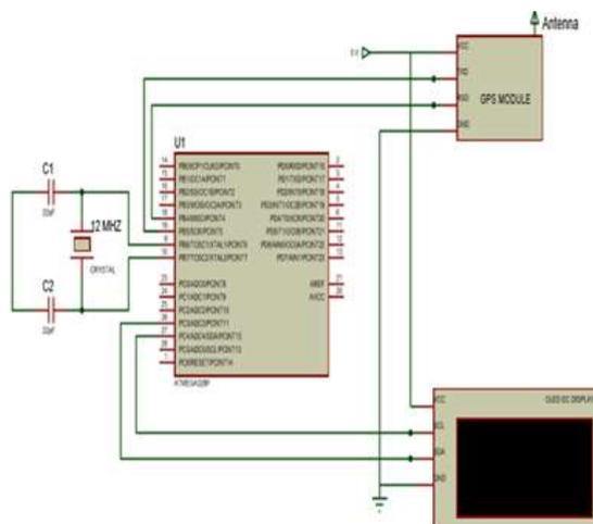
Fig 7: Circuit Diagram of the Auto-update Digital based watch system
