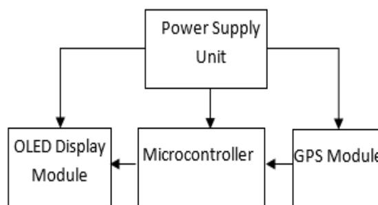
**Fig 1:** Block Diagram of the Auto-update Digital Watch Based Location System
