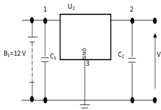
Fig 5: Circuit Diagram of the Power Supply Unit
