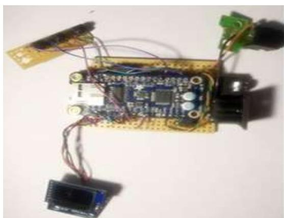
Fig 9: The Arrangement/Connections/Soldering of the Modules/Components on a Vero Board
