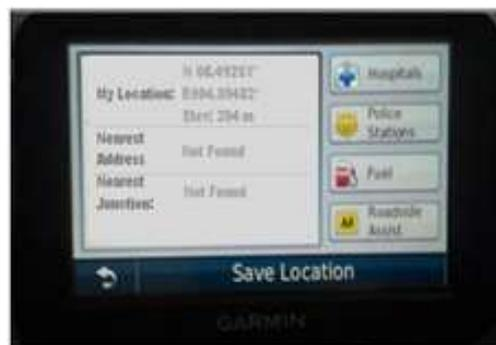
Fig 10: Standard GPS (Garmin-nuvi 40GPS) Location co-ordinate at the Same Location and as Time as that of Figure 9.
