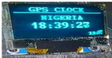
Fig 11: The Display of the Local Time on the Developed Digital Based Location System at one of the Test Location
