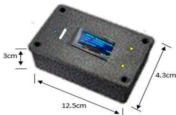
Fig 10: The Picture of the System Casing.
