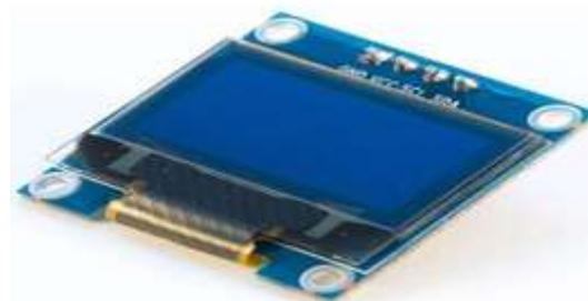
**Fig 2:** Picture of the 0.96 in, 64 X 128 OLED Display Module
