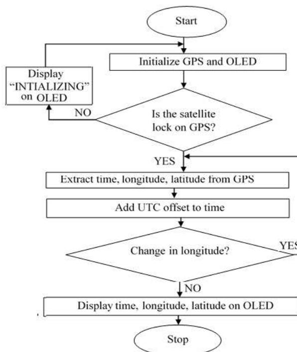
Fig 6: Flowchart of the Auto-update Digital based watch system
