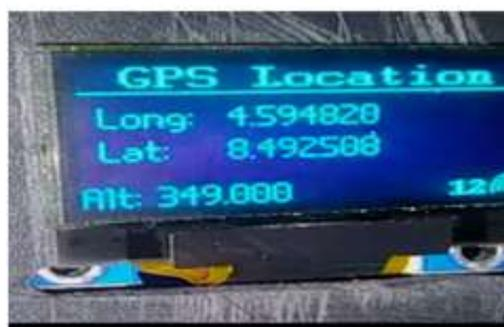
Fig 9: The Display of the Location Co-ordinate on Developed Digital Based Location System at One of the Test Location
