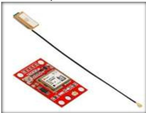
Fig 3: Picture of the Neo-6M GPS
