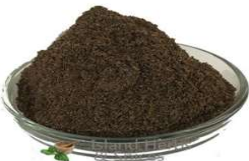
Fig 3: Papaya seed grinded into powder use for surface water treatment
