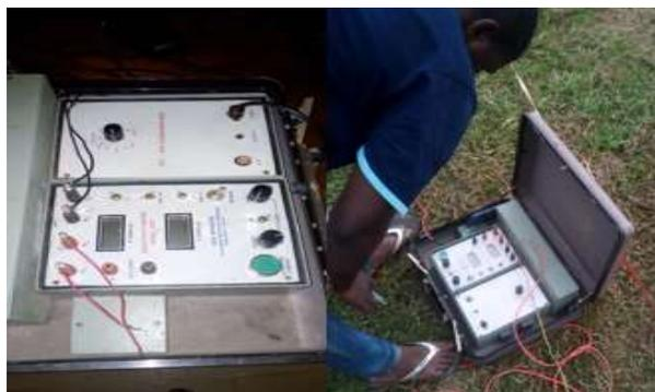
Fig 1: Geo sensors resistivity meter used for data gathering.
