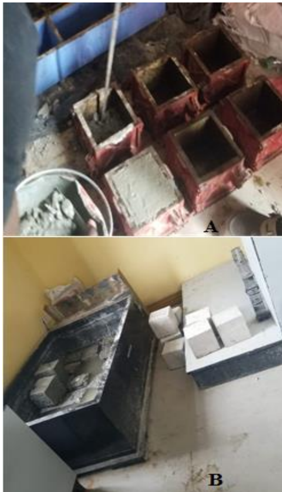
Fig 2: Laboratory Procedure Showing Casting Molds (A), Casted Cubes (B) and Curing Tank (B)
