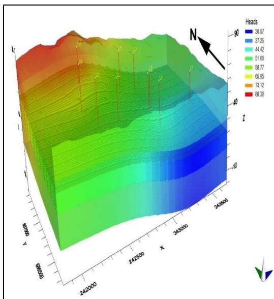
Fig. 3: Oblique view of groundwater flow in the region.
