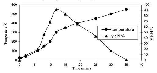
Fig 3 Effect of Temperature and time on the yield of gaseous products
