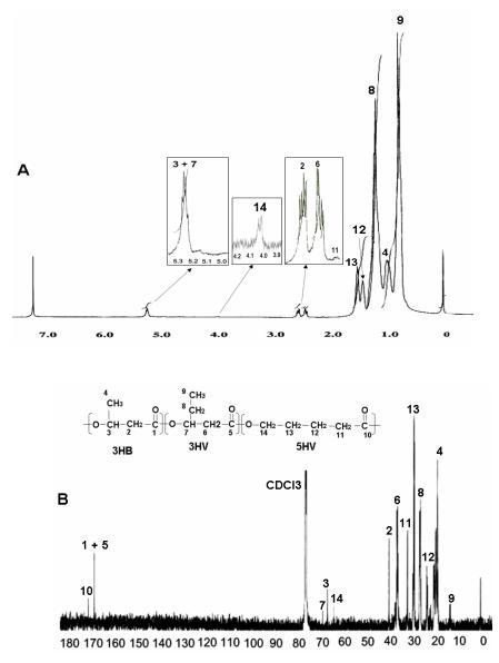
Fig 3:  $^1\mathrm{H}$  NMR (A) and  $^{13}\mathrm{C}$  NMR (B) spectra analysis of the polymer produced by the wildtype yeast strain RY4
