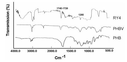
Fig 2: Infrared-spectra (IR) of PHA: Standard PHB; Standard PHB-co-PHV; PHA polymers produced in strain RY4.
