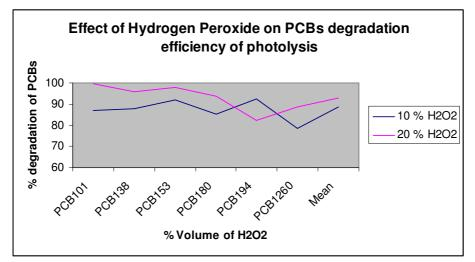
**Figure 2:** Effect of Hydrogen Peroxide on PCBs degradation (%) of photolysis: *Experimental conditions: Volumes of ethanol and transformer oil* (1:1, 2:1, 3:1),  $pH=7\pm0.5$ , *Temperature=*  $34 \pm 1.5$ , *exposure time=* 6 *hour*
