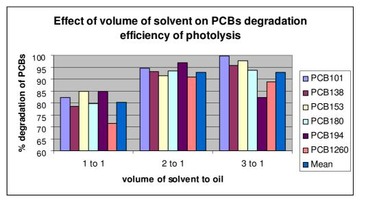
*Experimental conditions: Volumes of ethanol and transformer oil (1:1, 2:1, 3:1), pH=*  $7\pm0.5$ , *Temperature=*  $34\pm1.5$ , *exposure time=* 6 *hour*
